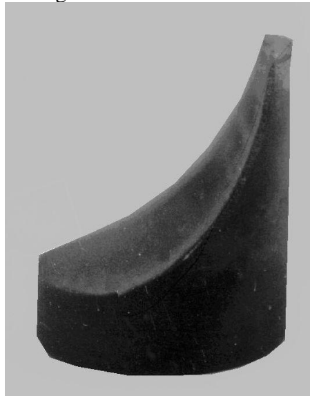
Fig.1 - Construction of a refractor for blast-holes setting down on a contour
