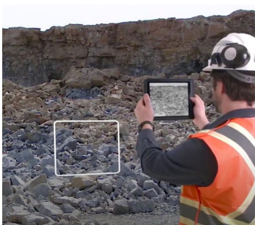
Figure 1 – Field photo analysis of rock fragmentation using tablet-based image capture
