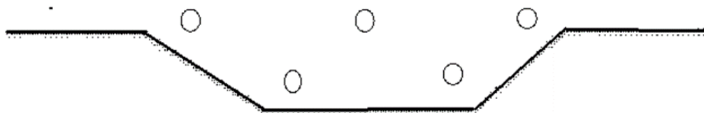
Figure 1 – A typical face to be blasted of firing for holes
